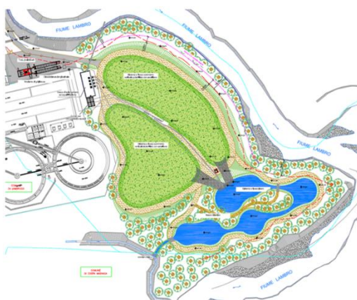
Figure 1. Treatment wetland at the municipal wastewater treatment plant in Merone, Italy. Source: Rizzo, 2022.
