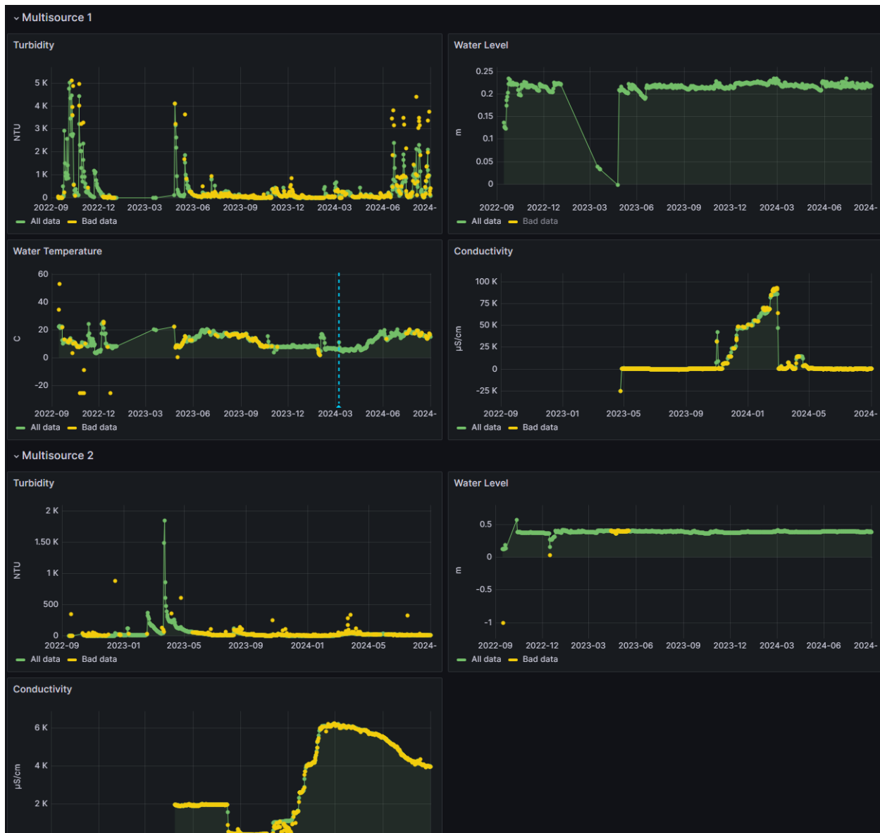
Figure 7.3 Overview of the sensor monitoring data from the inlet (Multisource 1) and the outlet (Multisource 2) for the parameters turbidity (NTU), water level (m, only for inlet), water temperature (Co) and conductivity (µS/cm) over the complete project period October 2022 - September 2024.
